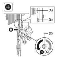
Turn the top adjustment bolt to adjust so that the guide pulley is below the outer line of the smallest sprocket when viewed from the rear.
