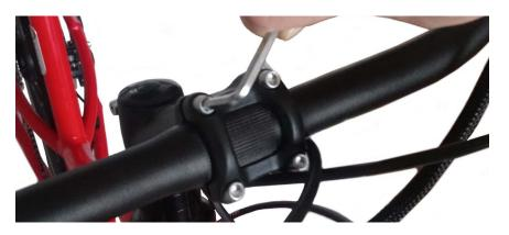
Make sure that the bolts are all evenly tightened, and that there is an even gap on the top and the bottom of the stem faceplate. Ensure that the handlebar is perfectly centred and set to the desired angle.
