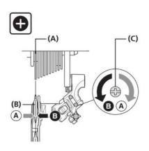
Turn the low adjustment bolt so that the guide pulley moves to a position directly in line with the largest sprocket.
