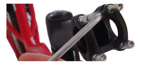
Place the knurled part of the handlebar into the stem faceplate and tighten the screws with an Allen key.
